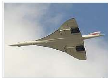
The Concorde supersonic transport had an ogival delta wing, a slender fuselage and four underslung Rolls-Royce/Snecma Olympus 593 engines.
