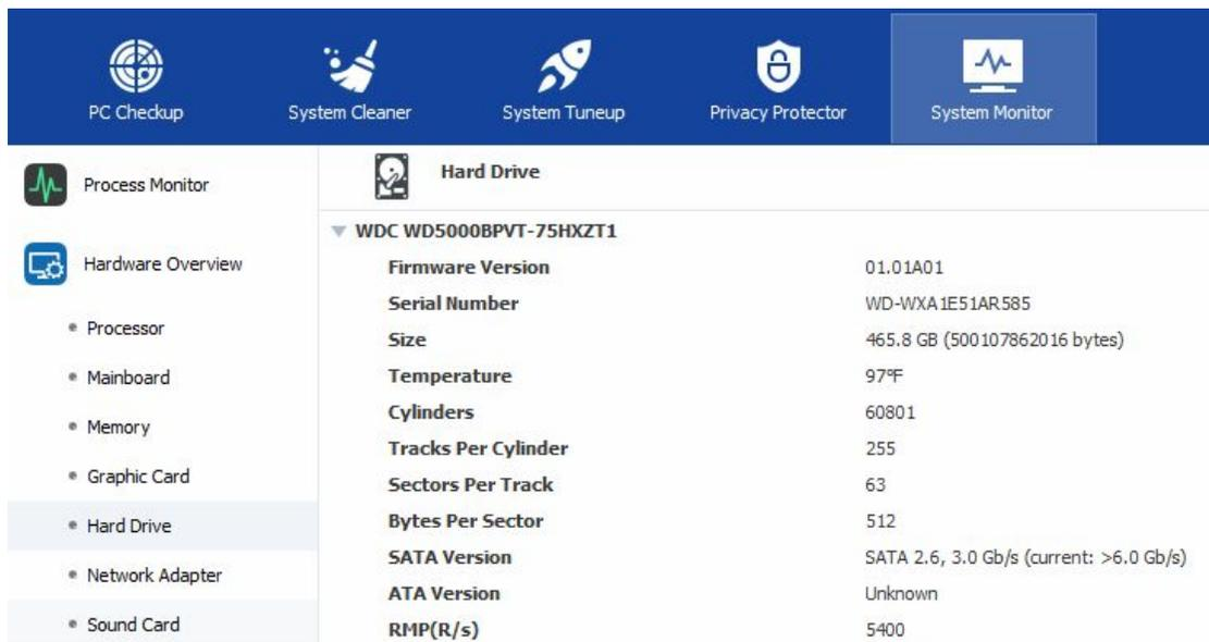
System Monitor displays many details of the computer it is being run on.
